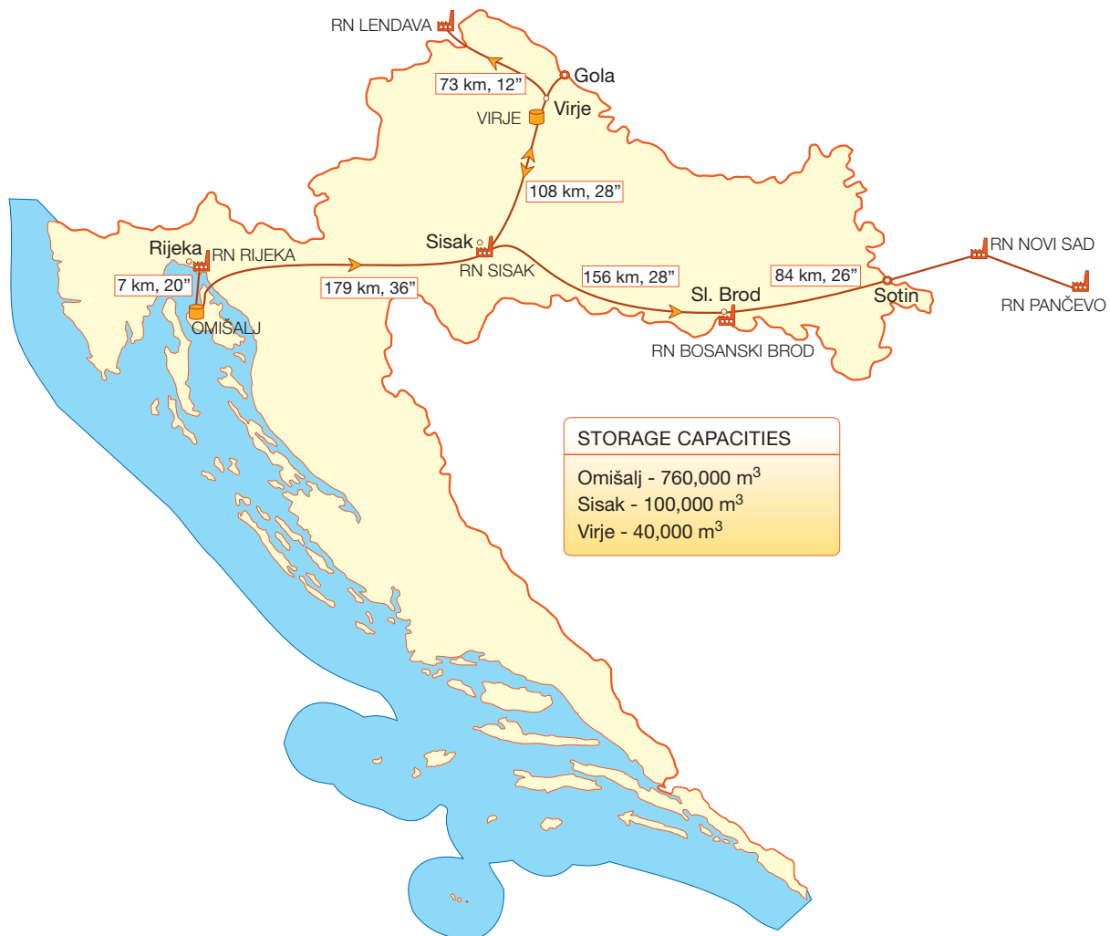
Picture 36: JANAF d.d. transport system for supply of refineries in Croatia and in neighboring countries, with oil pipeline routes and tanker and storage capacities
