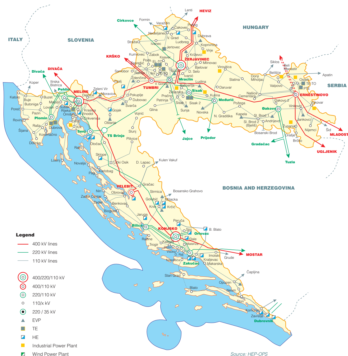
Figure 3.1.1. Scheme of transmission network and production facilities of the Croatian electric power system
