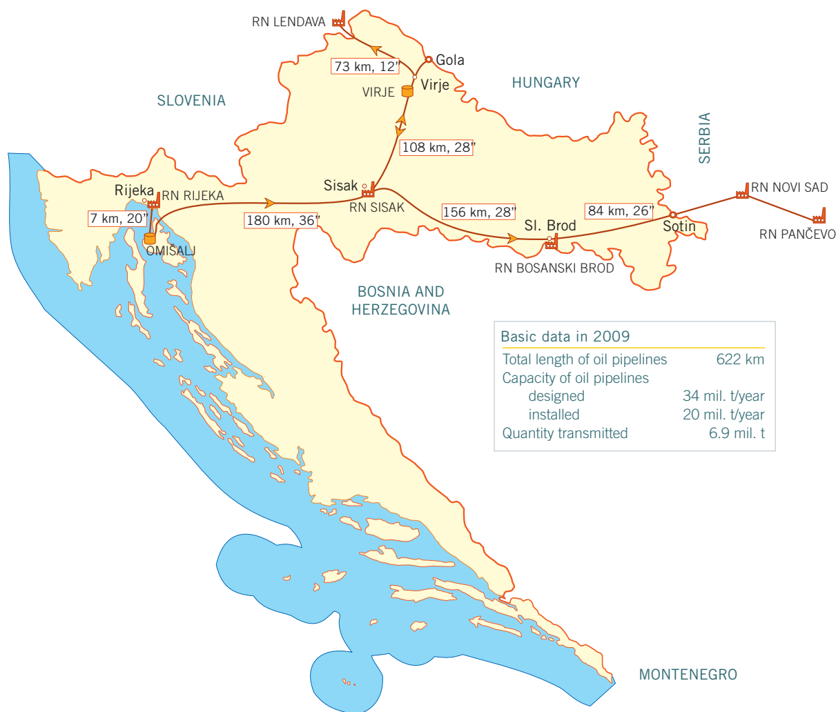
Figure 5.1.1. JANAF d.d.'s oil pipeline system
