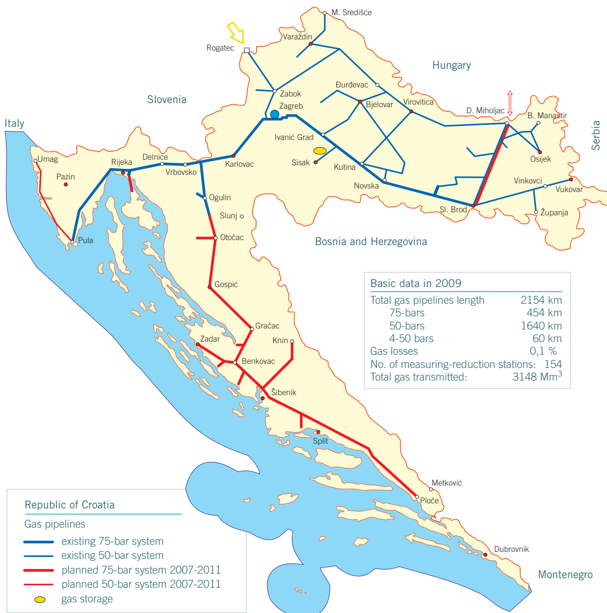
Figure 4.1.1. Existing and planned gas transmission system of the Republic of Croatia
