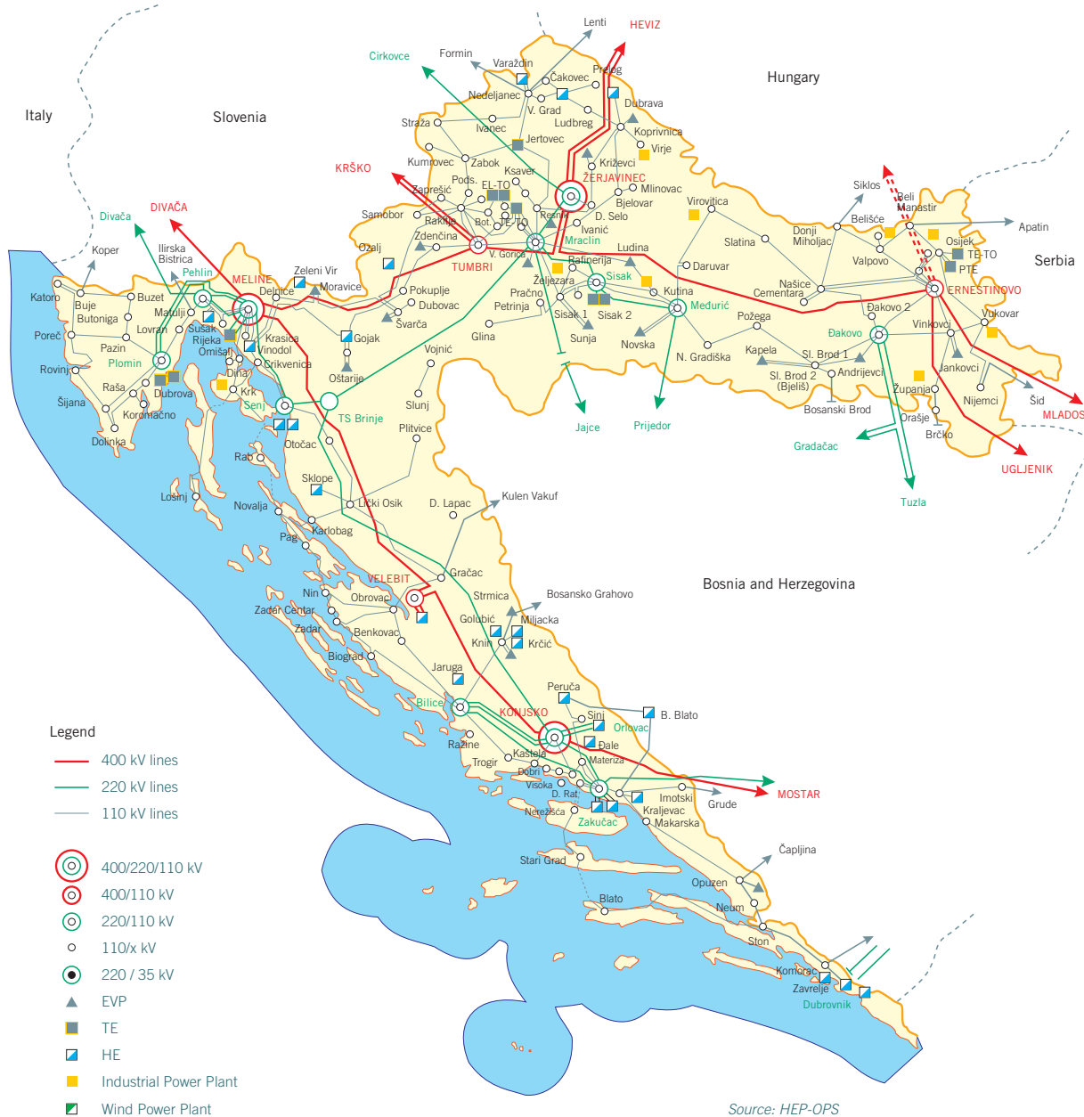
Figure 3.1.1. Scheme of transmission network and production facilities of the Croatian electric power system
