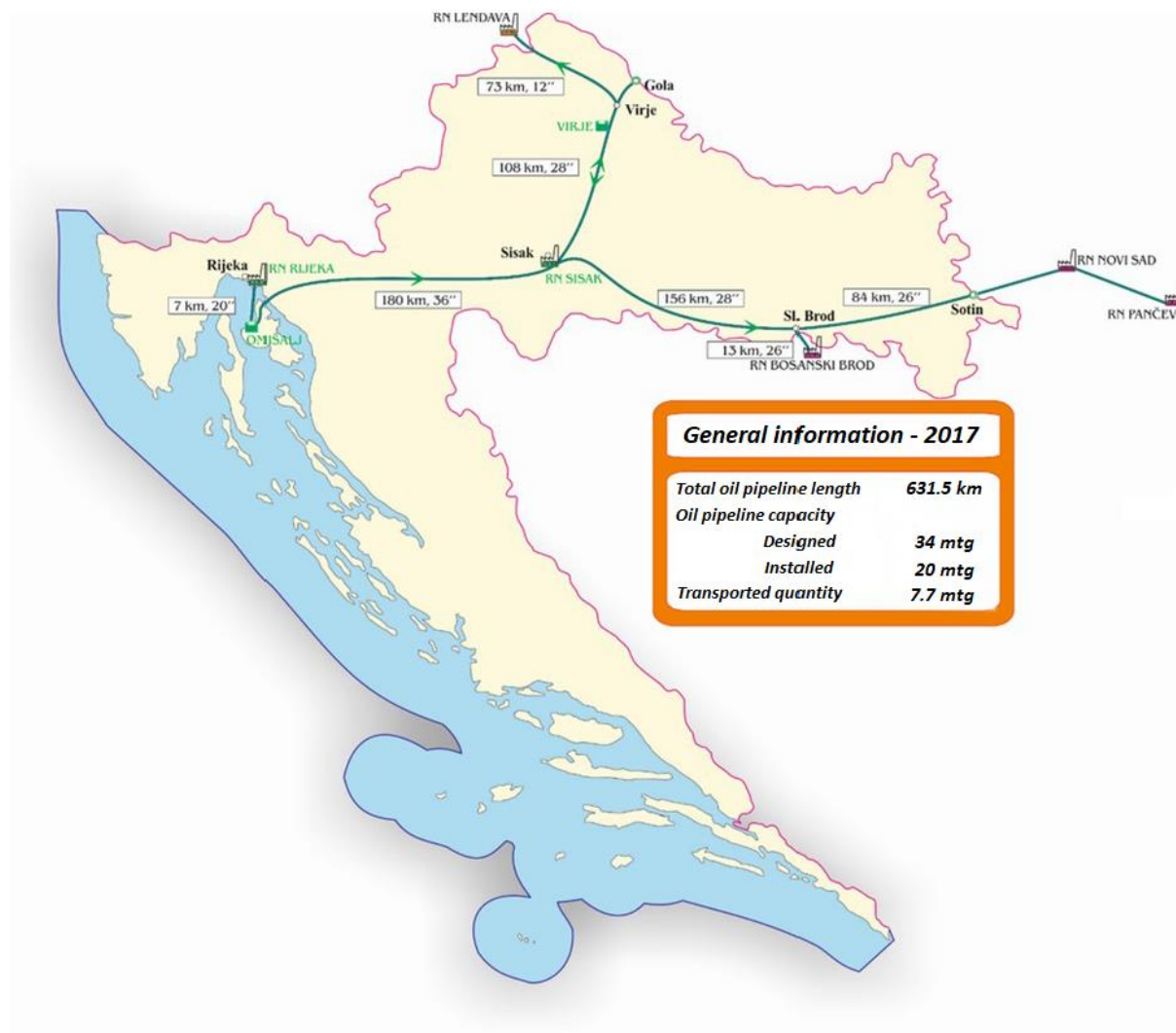
Figure 6.2.1 JANAf d.d. oil pipeline system
