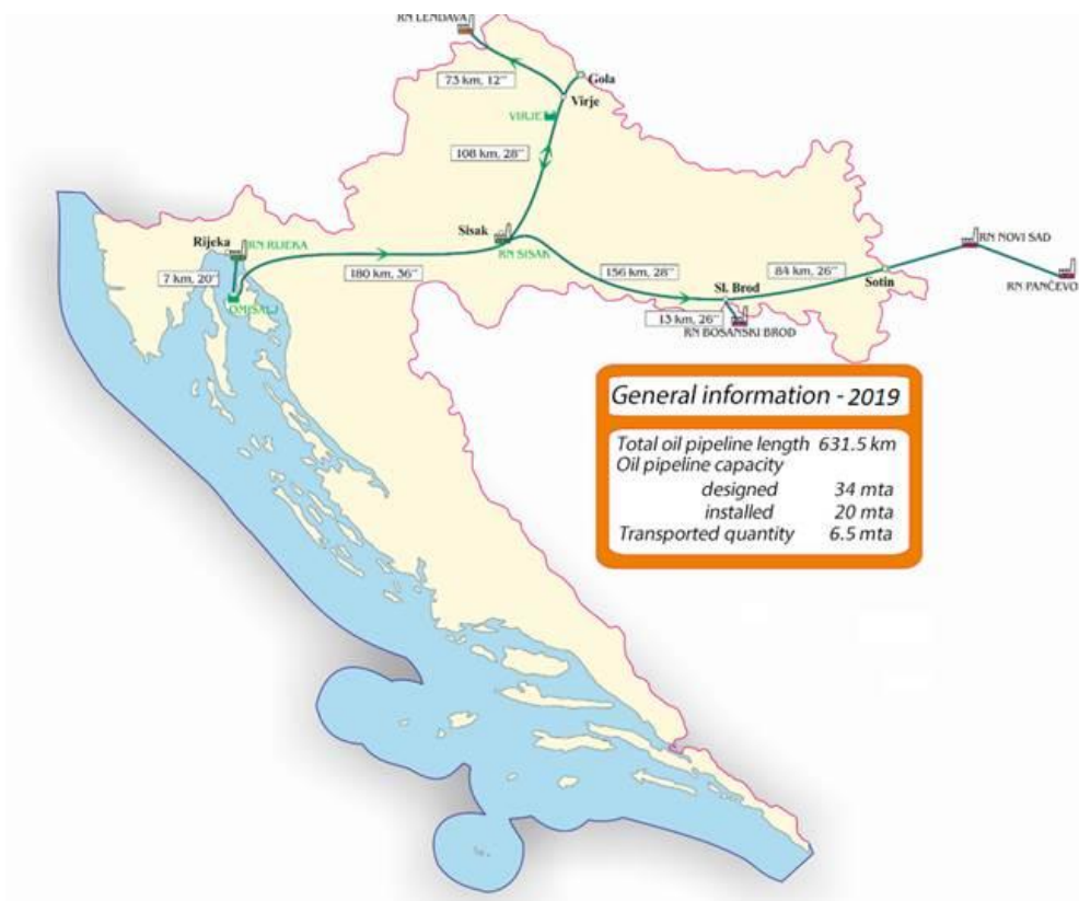
Figure 6.2.1. The JANAF d.d. oil pipeline system
